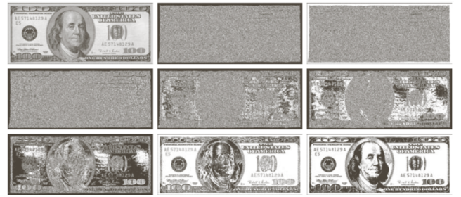
Fig. 10. Bit-plane slicing on a 100$ bill
